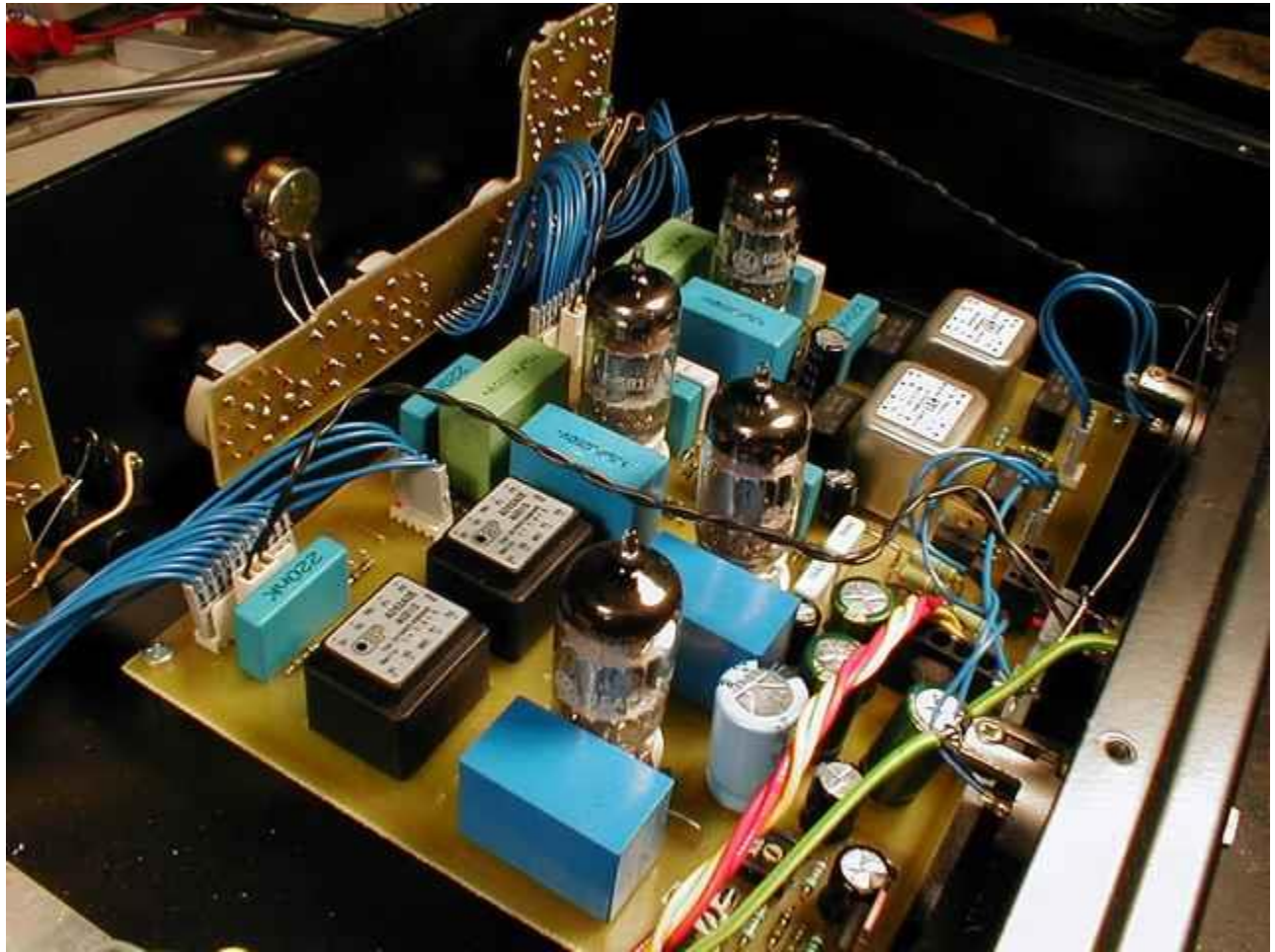
The main PCB and one control PCB..
